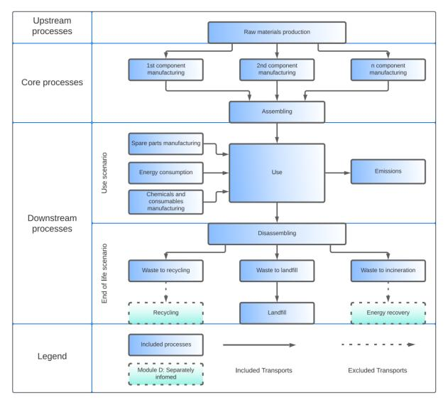
Figure 10: System diagram illustrating the processes that are included in the product system, divided into upstream, core and downstream processes., based on PCR Other special-purpose machinery.
