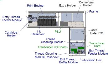
Figure 4, show side view drawings of the Coloreel unit.
